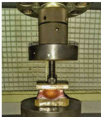
Figure 10 Model palced on UTM table with screw in between the slab and mandrel.
