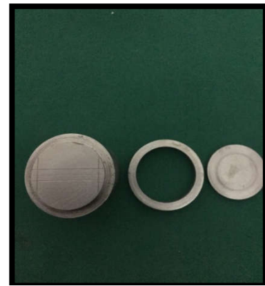
Fig 2 Master die with riser
