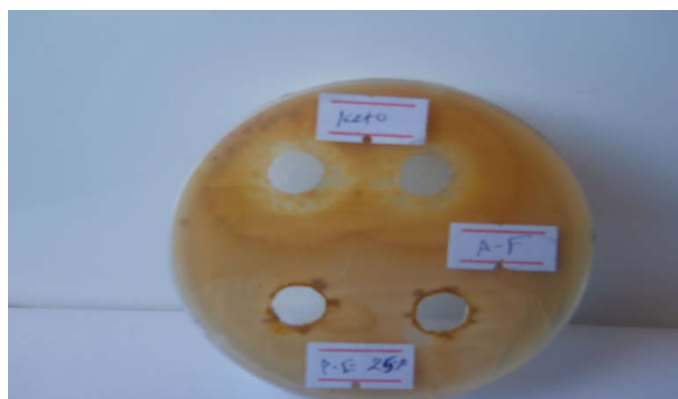
Plate (2) displays zone of growth Inhibition Aspergillus flavus using P.E.E. conc. 25% compared with the Control ketoconazole.
