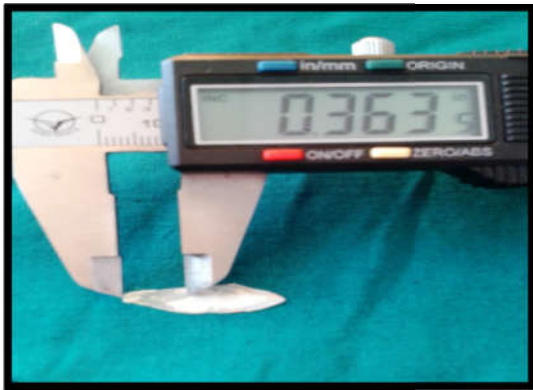
Figure 1 Length wise reading taken with help of digital calliper for digital method
