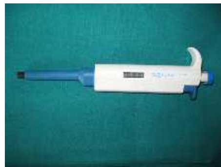
Fig 2 Micropipette used for pipetting of blood sample
